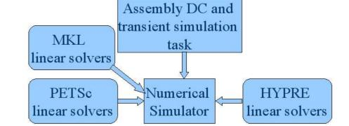
Figure 2: Components of implemented parallel power grid simulator
